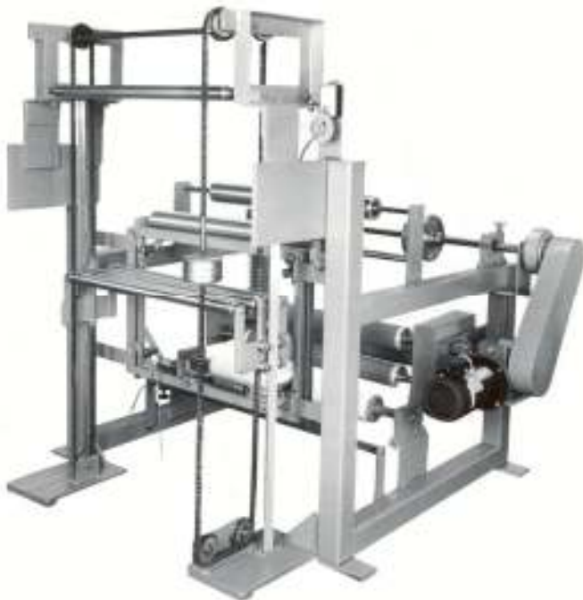
SINGLE STATION REWIND STAND with "S" WRAP FEED ROLLS and ACCUMULATOR ASSEMBLY
