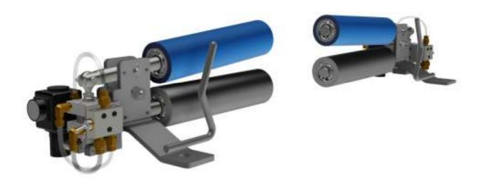
The Air loaded Adjusta-Pull assemblies are easy to open and close which allows fast and easy web threading and include a pressure regulator to accurately adjust the air pressure to accommodate all types of material including delicate webs. They can be designed to allow remote open and close functionality.
