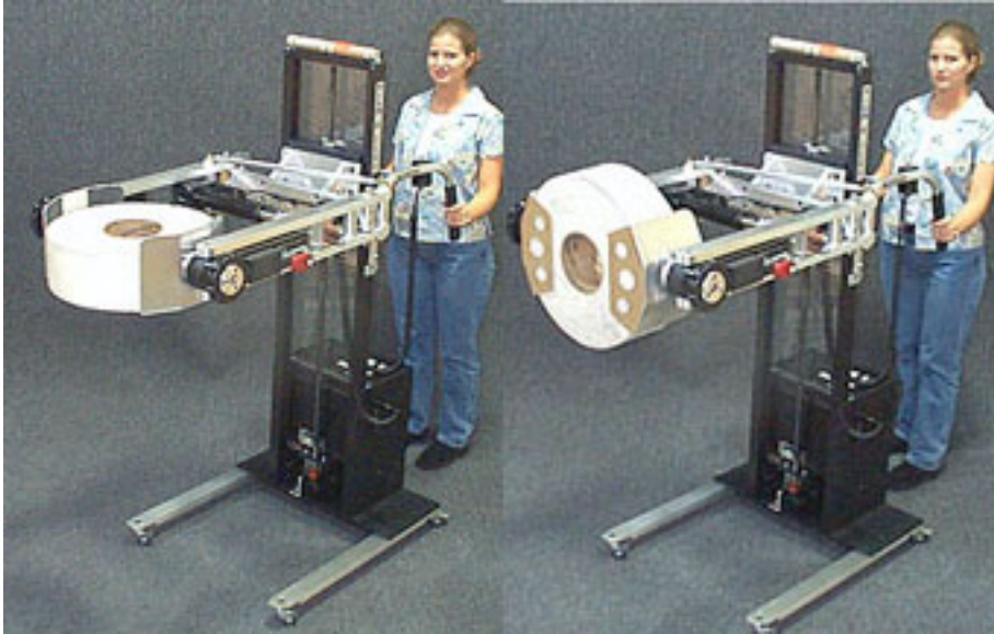
THIS WALK-BEHIND WITH ROLL CLAMP HAS ANTI-TELESCOPING FLANGES
