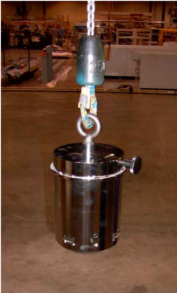
CORE PROBE FOR LIFTING AND MOVING PERPENDICULAR ROLLS (THIS UNIT IS NOT DESIGNED TO TURN ROLLS).
