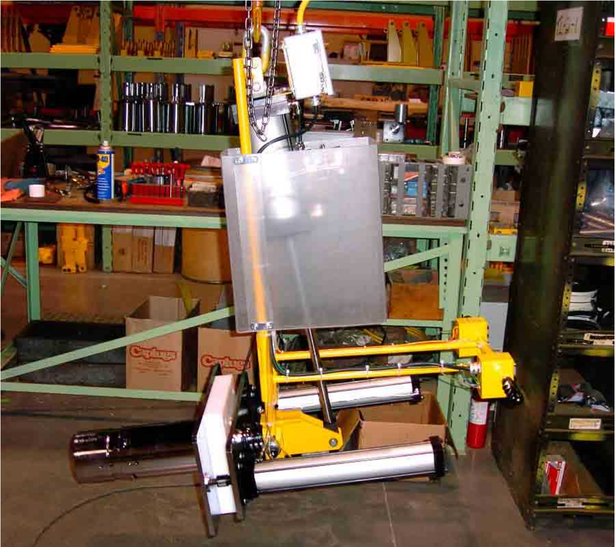
OVERHEAD ROLL HANDLING SYSTEM FOR USE WITH SINGLE HOIST. THIS UNIT INCLUDES SHAFT LOADER.
