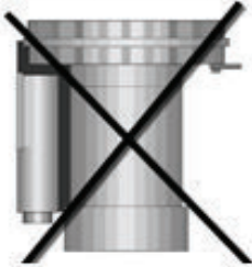
Incorrect Vertical Position
