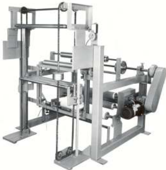
SINGLE STATION REWIND STAND with "S" WRAP FEED ROLLS and ACCUMULATOR ASSEMBLY
