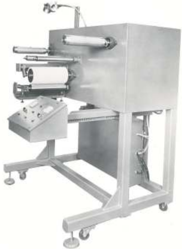
CANTILEVERED SPECIAL UNWIND / REWIND STAND
